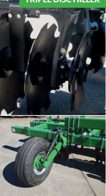
The Gessner Triple Disc Hiller is designed to provide an effective solution for building and renovating beds in rowcrop applications. The unique design of triple disc hiller units ensures effective trash and chemical incorporation in various tillage applications. Triple Disc Hiller units may be purchased in individual pairs or as a part of a complete machine.
