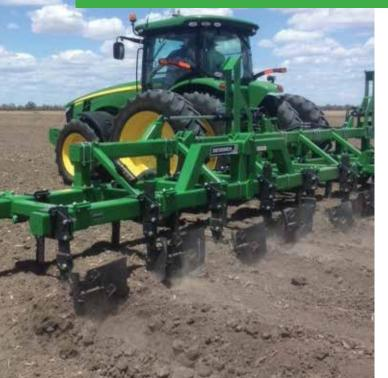
Gessner Centre Busters are designed to provide a highly effective solution for a wide variety of row-crop tillage applications. Featuring a durable, field-proven frame design in widths ranging from 4 row to 12 row and hard-wearing customisable attachments, Gessner Centre Busters are fully equipped to cater for all of your row-crop and dryland tillage requirements.
