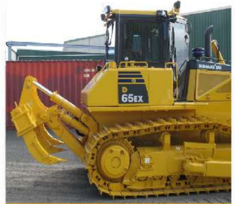
VARIABLE PITCH RIPPER — KOMATSU D65
