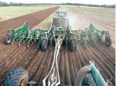
The Gessner Landmaster can be configured to suit a range of applications, catering for all of your Broadacre planting requirements. Standard Landmaster configurations range from 12m to 24m featuring tyne spacing ranging from 333mm to 500mm. In addition, custom configurations are available to ensure that all of your planting needs are catered for.
