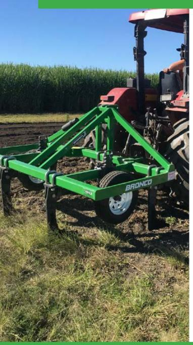
Ideally suited for smaller horsepower tractors the Gessner Bronco is a reliable and well designed deep ripper that will suit those farmers with smaller acres requiring a primary till. Standard tyne spacing is 500mm for both the 5 and 7 shank models. However, custom machine sizes and various tyne configurations are available to suit all customers requests. Hook the Gessner Bronco on and off your tractor in minutes.
