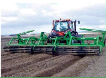
The Gessner Offset Disc Plough has been designed to provide heavy duty ploughing capabilities for sugar cane stubble management. The plough is available in a range of disc number configurations, spacings and weights to cater for all of your heavy duty sugar cane tillage requirements. Prepare your country with confidence with a Gessner Offset Disc Plough.
